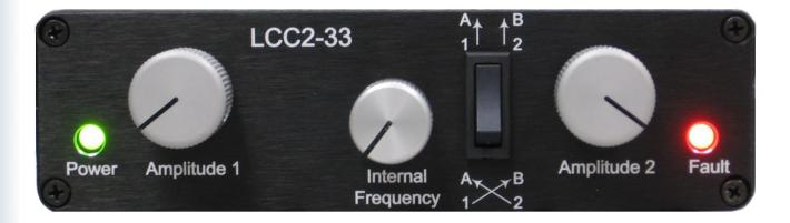
The **LCC2-33** is a versatile dual-channel liquid-crystal controller, designed to run continuously-variable liquid crystal (LC) devices such as variable retarders, polarization switches, shutters, attenuators, and tunable color filters. LC voltages up to 33  $V_{\text{RMS}}$  are controlled by two amplitude knobs.
